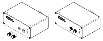
Security Cover Installation - Remove the knob from the panel and insert the cover. Small
