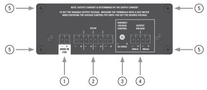
TSD input / output connections are removable for easy system wiring. The connector has a 3.5mm pitch between pins.
