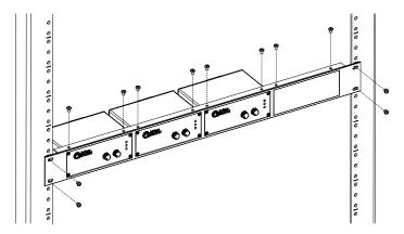
2. TSD-RMKHR Half Width Rack Mount Kit - AtlasIED offers an optional rack mount kit that can be used in half width rack applications including the AtlasIED WMA-HR and AWR-HR models. The TSD-RMKHR can support up to two TSDs. Included is an extra blank panel to fill one of the spaces if only one TSD is being used.
